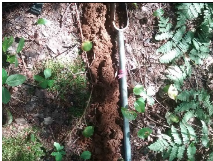
Photo 1: Coarse, mineral soils identified using a hand auger in the field
